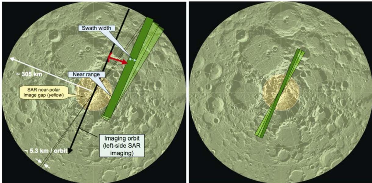
Figure 5. Nominal SAR and scatterometry polar mapping strategy.
