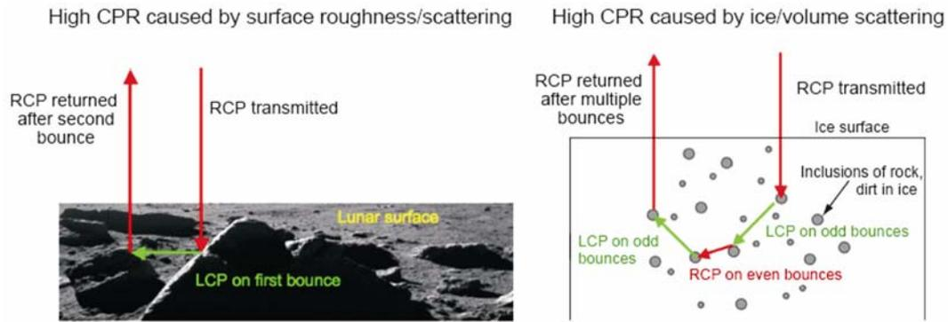
Figure 1. Elevated circular polarization ratio caused by ice (volume) or roughness (surface) scattering (from Spudis<sup>10</sup>).
