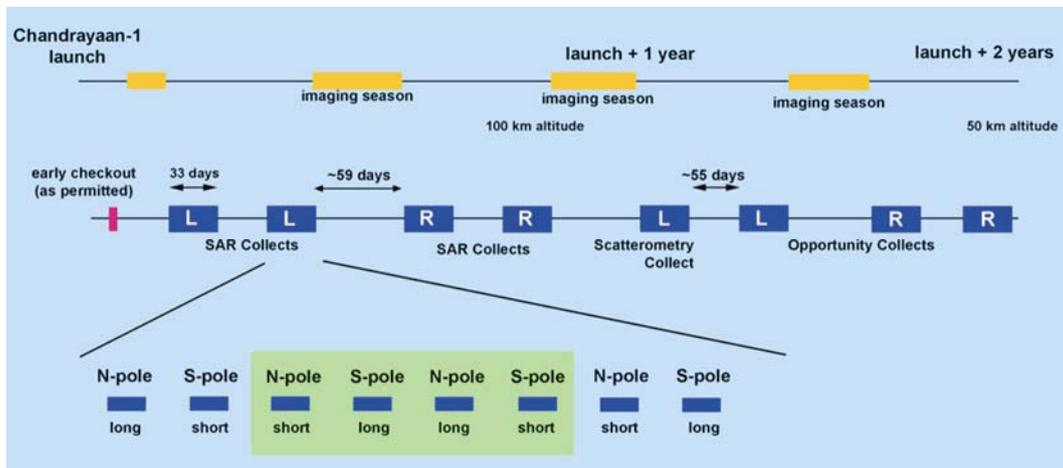
Figure 4. Chandrayaan-1 Mini-SAR measurement timeline.
