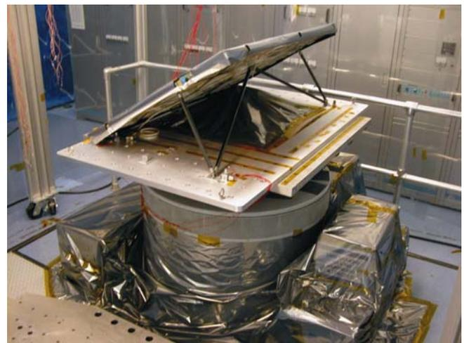
Figure 7. Mini-SAR antenna during testing.
