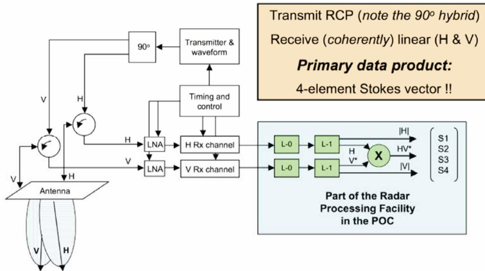
**Figure 2.** Block diagram of Mini-SAR, showing the hybrid polarity architecture used to gather information on lunar surface Stokes parameters.
